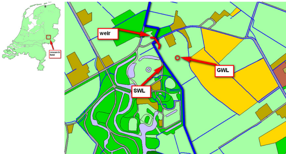
Figure 12.7 Location of monitoring site at the Wildenborch estate where groundwater levels (GWL) and surface water levels (SWL) were measured and controlled by a weir.
